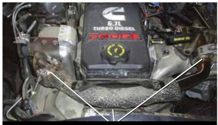
Loosen clamps on both sides of the EGR crossover pipe. Remove 1x 8mm bolt in the center of the pipe (underneath).
