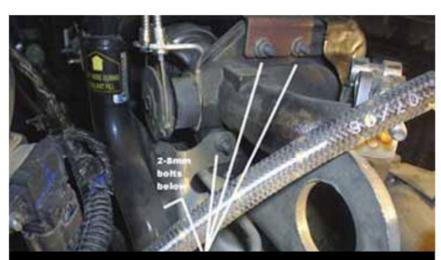
Remove 3x 10mm nuts and 2x 8mm bolts. Remove heat shield.
