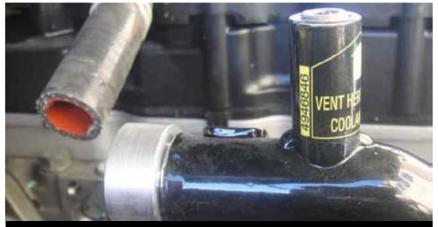
Install coolant plug into coolant pipe. It is recommended that you apply a thin coat of lubricant on the o-ring before installation. Ensure that the plug is pressed all the way in.
