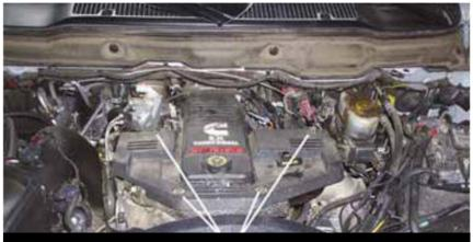
Remove 4x 8mm bolts. Remove dipstick and plastic cover.
