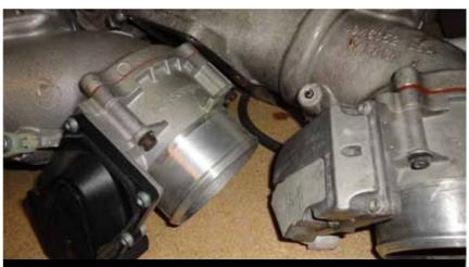
Unplug EGR airflow valve (shown here with intake manifold removed for better picture).
