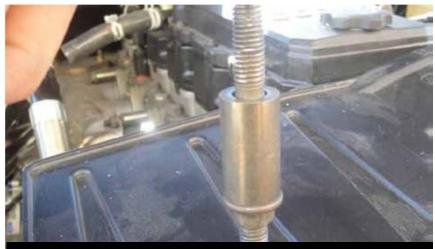
Remove spacer from previously installed header bolt and install spacer on supplied header stud.
